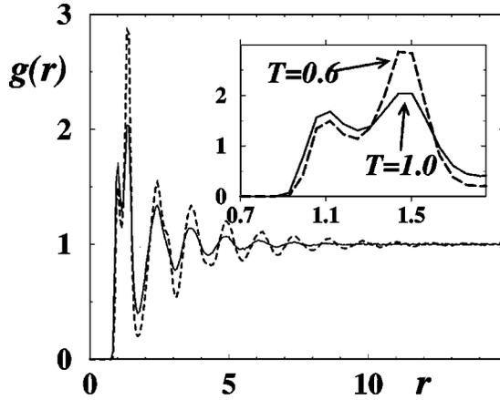
FIG. 4. Radial distribution function at high and low temperatures, along the  $P=0.48$  isobar for the smooth potential. Notice how, by lowering  $T$ , long-range correlations develop [ $g(r)=1$  if particles at distance  $r$  are uncorrelated] and more particles are expelled from inside the soft core  $r\sim 1.1$  into the attractive well  $r\sim 1.5$  (inset). As the average interparticle distance is growing upon cooling, the system is expanding and there is hence a density anomaly.
