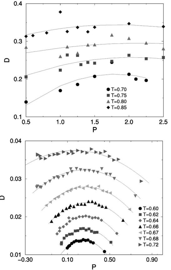
FIG. 10. Diffusion coefficient  $D$  in the liquid phase for the continuous potential (left panel) and the discrete potential (right panel) along various isotherms. Lines are intended as a guide for the eye. Notice the anomalous sections of the graph, where  $(\partial D / \partial P)_T > 0$ .
