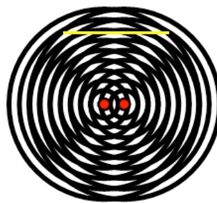
Figure 25.25: An interference pattern set up in a room by two speakers broadcasting identical single-frequency waves. For Exercise 4.
