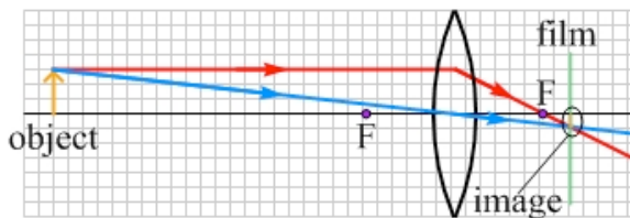
Figure 24.44: In a camera, the lens has a fixed shape, so the lens is moved to the right, closer to the film, when the object is moved farther from the camera. This produces a focused image on the film.
