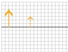
Figure 24.65: The larger arrow represents an object, while the smaller arrow represents the virtual image of that object, created by a lens. For Exercise 47.
