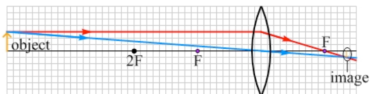
Figure 24.32: A ray diagram for the situation in which the object is far from the lens. The squares in the grid measure 1.0 cm × 1.0 cm.
