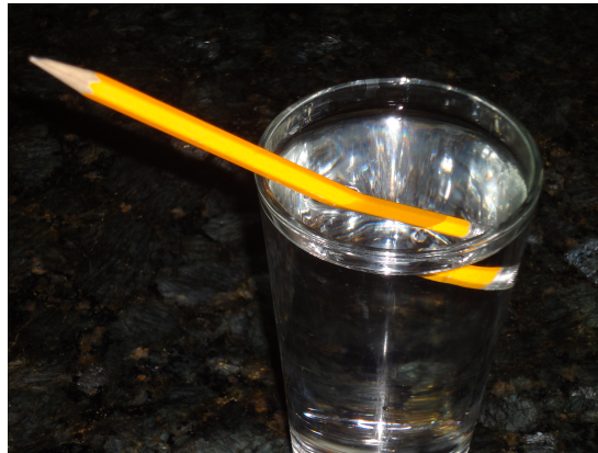
Figure 24.5: The photograph shows a picture of a pencil in a glass of water. Refraction of the light leaving the water makes the pencil appear to bend. Photo credit: A. Duffy.
