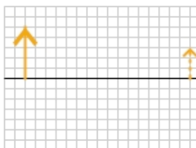
Figure 23.52: The larger arrow represents an object, while the smaller arrow represents the virtual image of that object, created by a spherical mirror. For Exercise 45.
