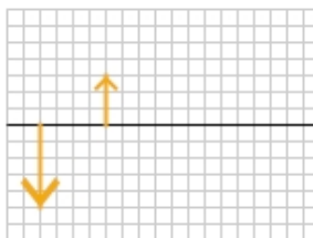
Figure 23.51: This figure shows an object and a real image created by a spherical mirror. For Exercise 44.
