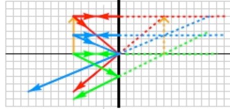
Figure 23.14: Compare this figure to Figure 23.12. Moving the object closer to the mirror moves the image closer to the mirror, but the height of the image is still equal to the height of the object.
