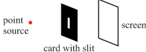
Figure 23.38: A point source of light illuminates a card with a narrow slit. For Exercise 3.
