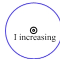
Figure 20.36: A long straight wire passes through the center of a conducting loop. The current in the long straight wire is directed out of the page, and is increasing in magnitude. For Exercise 5.
