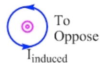
Figure 20.16: To oppose the change in flux as the loop moves from Before to After, the loop creates a magnetic field out of the page with a counterclockwise induced current.
