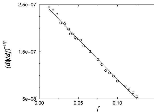
FIG. 3. The susceptibility  $d\phi/df$  for the spring network of size  $L = 50$ , averaged over  $N = 100$  configurations, is plotted as function of the applied stress  $f$ . Mean-field scaling ( $\gamma = 1/2$ ) appears to be very good also in this case.
