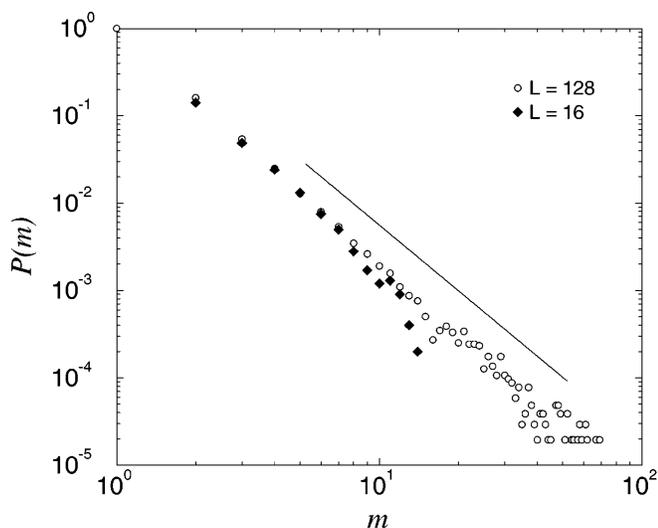
FIG. 2. The avalanche size distribution for a random fuse model of size  $L = 32$  and  $L = 128$  is plotted in log-log scale. A line with the mean-field value  $\tau' = 5/2$  of the exponent is plotted for reference. The cutoff of the distribution increases with the system size.
