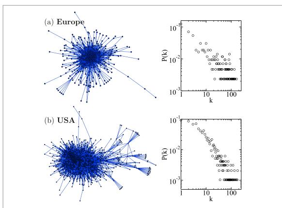
**Figure 8.** Real airline networks and their degree distribution for Europe (a) and USA (b), obtained from the Flightradar 24 data [41]. The sizes are: N=425 for Europe and N=973 for USA, and the number of links are: 5636 and 8724, respectively. The degree–degree  $(r_p)$  correlation and clustering coefficients (C) are:  $r_p=-0.14$  and C=0.59 for Europe, and  $r_p=0.09$  and C=0.30 for USA.
