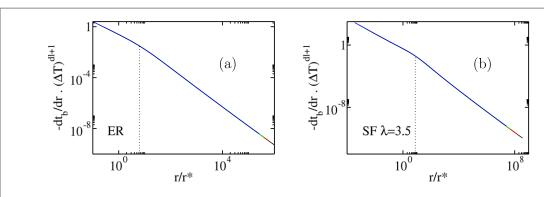
**Figure 5.** Collapse of the curves  $dt_b/dr$  as a function of r. (a) ER network with  $\langle k \rangle = 4$  for T=0.250 625 (black), T=0.250 78 (red), T=0.250 976 (green) and T=0.251 2207 (blue). (b) SF network with  $k_{\min}=2$  and  $\lambda=3.5$  for T=0.269 325 (black), T=0.269 481 (red), T=0.269 92 (green), and T=0.270 226 (blue). The dotted line indicates the position of the crossover. The figures are in log–log scale.
