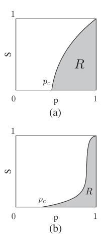
FIG. 6. Schematic profiles of the giant component as a function of the remaining node fraction, p, for the two typical cases. The case (a) has a larger value of the critical node threshold  $p_c$  than (b), but the giant component collapse for (a) occurs much slower than for the case (b). From the viewpoint of the global connectivity, the value of the area below S(p) represented by R is a better measure of the robustness than the critical threshold  $p_c$ .
