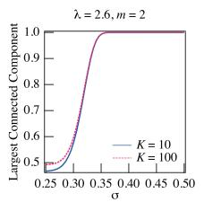
FIG. 3. (Color online) The fraction of the largest connected component of scale-free networks with the exponent  $\lambda=2.6$ , minimum degree m=2, and maximum degrees K=10,100 as a function of the parameter  $\sigma$ , that controls the assortativity of the degree-degree correlation. Above  $\sigma\approx0.35$ , the separated k=2 components become connected to the larger degree components and the largest connected component spans the entire network.
