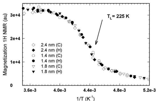
Fig. 7. NMR measurements of magnetization  $M_0$  versus inverse  $T$  of hydrated lysozyme in MCM nanopores of three different diameters (1.4 nm, 1.8 nm, and 2.4 nm) measured upon cooling (C) or heating (H).
