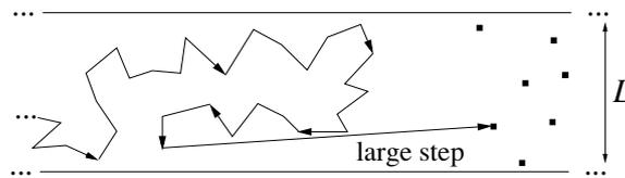
**Figure 7.** Deterministic search walks in rectangular environments with randomly distributed targets, where the ‘go-to-the-nearest-site’ rule leads to power-law distributions of move lengths for specific critical aspect ratios for  $L$  (strip-like geometry). This surprising result is due to the fact that in the critical condition the walker can ‘accidentally’ back track, and ends up having to make an ultra-long flight to return to the forward more abundant region of target sites [65].
