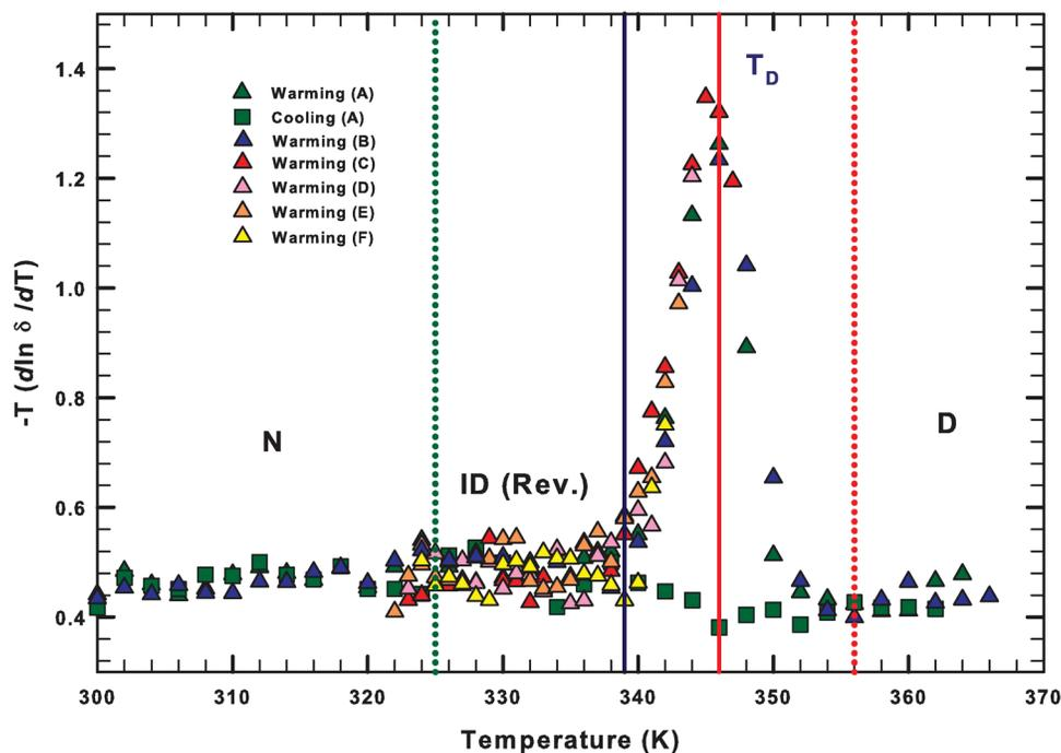
**Figure 9.** The configurational specific heat evaluated according to the procedure described in eq 3 for all the cycles during the warming phase. The cooling part is reported only for cycle A for simplicity. It is worth noting that the value of the obtained maximum is, within experimental error, the same as that measured by the DSC and TMSC calorimeters.<sup>27</sup>
