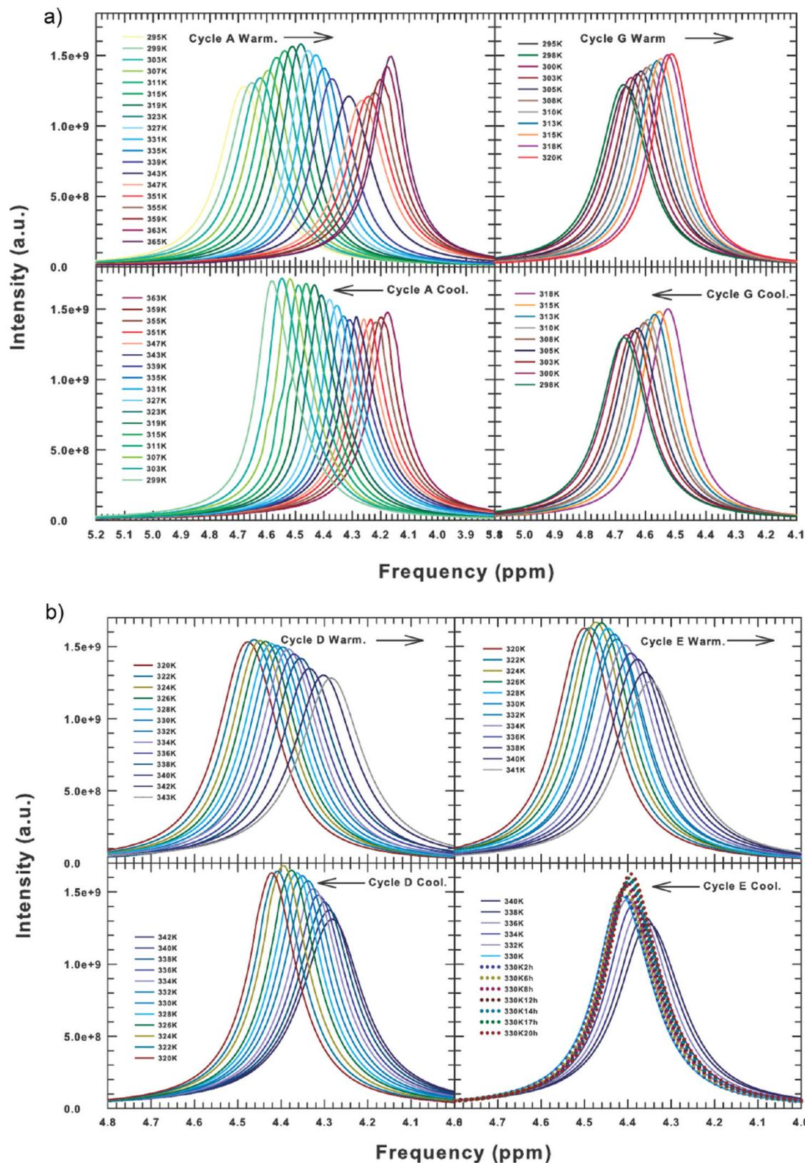
**Figure 4.** The thermal evolution of the NMR signal of the water protons during some characteristic warming–cooling cycles. (a, left side) Cycle A covers all three thermal regions: N, ID, and D; (a, right side) cycle G works only in the protein native region N; (b, left side) cycle D starts from 320 K up to 343 K and cooling back; (b, right side) cycle E starts from 320 to 340 K and cooling back up to 330 K where we have performed a PCS measurement with intervals of 1 h up to 20 h.
