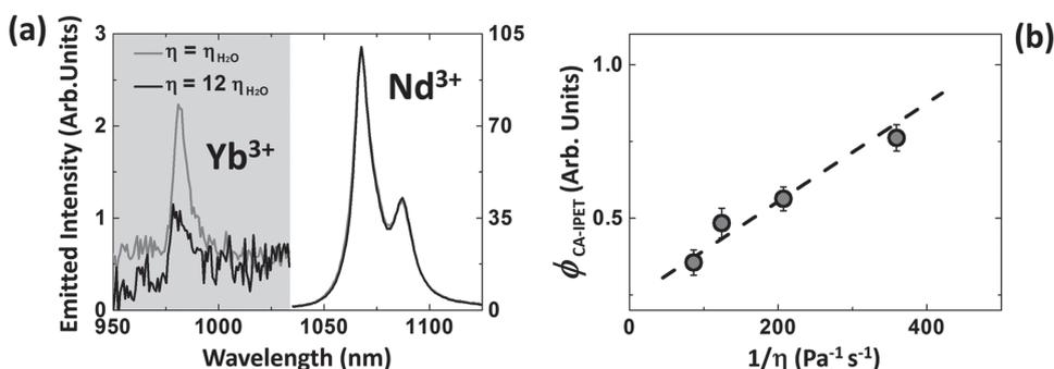
**Figure 2.** Dependence of IPET efficiency on viscosity. a) Emission spectra of the mixed LNF under optical excitation at 808 nm (i.e., optical excitation of doped SLNP:Nd) as obtained for two different viscosities of the solvent. b) Dependence of the CA-IPET efficiency on the inverse of fluid viscosity  $\eta$ . Symbols are experimental data and dashed line is a guide for the eyes.
