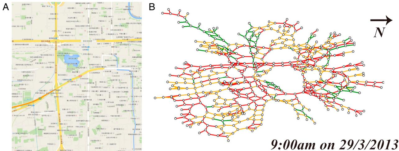
**Fig. 1.** Road network of the observed district. (A) Map of the investigated district. (B) Road network of the investigated district. Road network at 9:00 AM on March 29, 2013 is shown, where links are classified into three categories according to their velocity ratio  $r_{ij}$ : velocity ratio below 0.4 (red), between 0.4 and 0.7 (yellow), and above 0.7 (green). Note the clustering of each color.
