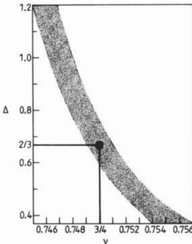
**Figure 1.** Dependence of the correction-to-scaling exponent  $\Delta$  on  $\nu$ , the 'trial' value of  $\nu$ , showing that even a very small change in  $\nu$  leads to a very large change in  $\Delta$ . The shaded region indicates the combination of several independent methods of estimating this dependence.
