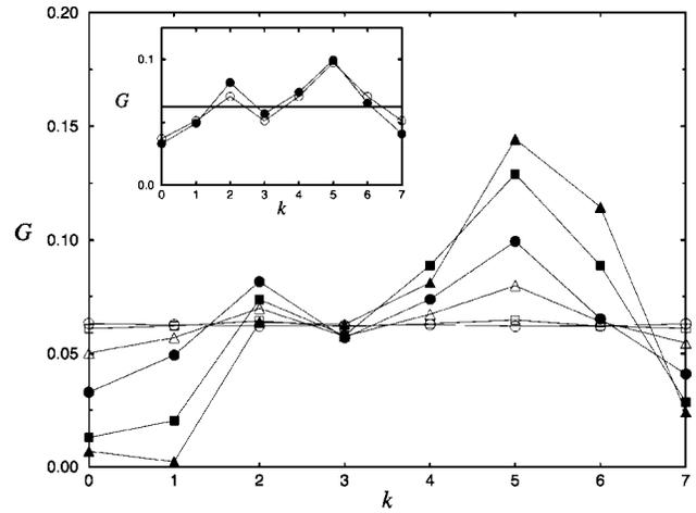
FIG. 6. Flux distributions  $G$  at the outlet branches in a five generation tree for  $Re = 150$  (circle), 300 (square), 600 (triangle), 1200 (full circle), 2400 (full square), and 4800 (full triangle). The inset compares the fluid flow simulations ( $Re = 1200$ , circle) and the binary tree model ( $p = 0.58$ , full circle).
