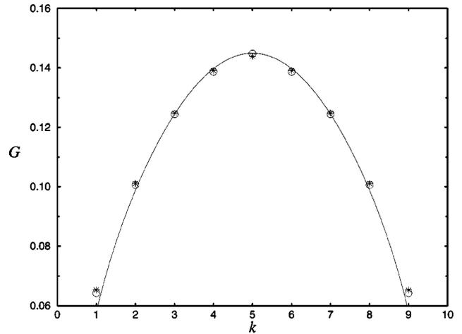
FIG. 13. Flux distribution at the outlet branches of a nine generation tree with loops for  $Re=1$  (circle). The results from an analog electrical network model (star) are in agreement with the fluid dynamic simulations. The solid line is the analytical solution of the infinite network [21].
