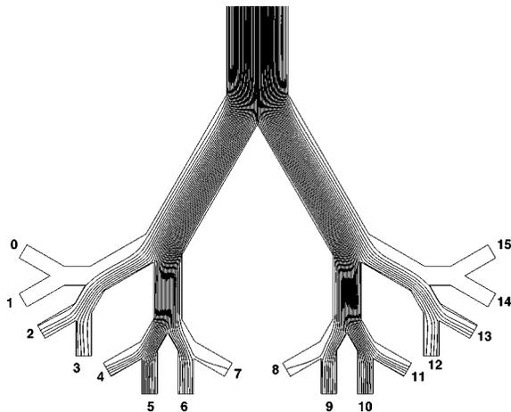
FIG. 5. Contour plot of the stream function in a five generation tree without loops for high Reynolds number conditions ( $Re = 4800$ ). The width of the first channel is  $d = 1.8$  cm and the length is  $l = 12$  cm.
