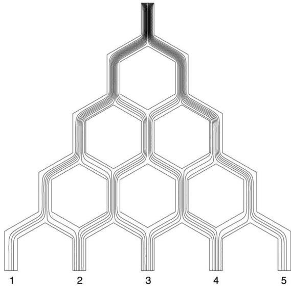
FIG. 12. Contour plot of the stream function in a five generation tree with loops. In this case, fluid is pushed from top to bottom throughout the tree at low Reynolds conditions ( $Re=1$ ). Note that the number of streamlines is larger (and thus the fluxes are higher) at the center channels in the last generation.
