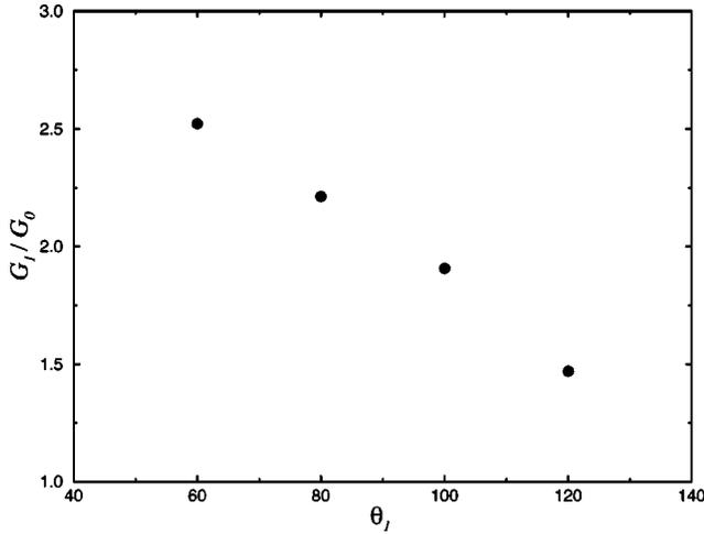
FIG. 8. Dependence of the flux ratio  $G_1/G_0$  on the bifurcation angle  $\theta_1$  between daughter branches at the second generation. The simulations have been performed with three generation trees at high Reynolds conditions ( $\text{Re}=1200$ ). The bifurcation angle at the second generation is  $\theta_2=120^\circ$ .
