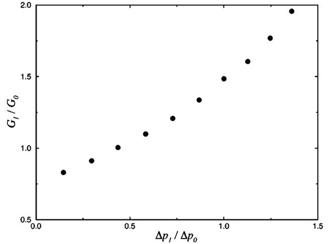
FIG. 9. Dependence of the flux ratio  $G_1/G_0$  on the pressure drop ratio  $\Delta p_1/\Delta p_0$  in three generation trees ( $\theta=120^\circ$  and  $\text{Re}=1200$ ).
