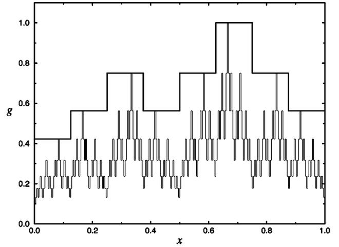
FIG. 11. Distribution of normalized fluxes  $g(x)$  defined in Eq. (5) as a function of the normalized branch number  $x$  at the outlets of a five generation (thick line) and a ten generation (thin line) tree. These steplike functions are calculated using the binary tree model with a partitioning ratio  $q/p=0.75$ .
